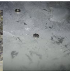
Removal of an adhesive/paper layer on a heat radiator in the paper industry
